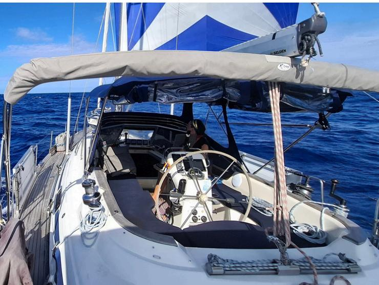
*The deck layout has been optimised for offshore liveaboard cruising, with the addition of a substantial davits arch, bow sprit, electric furling headsail winch, and both bow and stern thrusters.*
