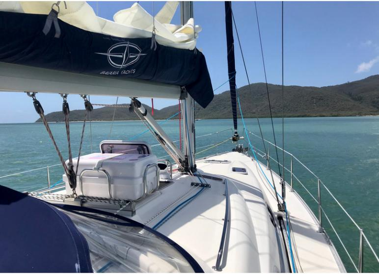
*Fandango has sleek lines, an open transom with sugar scoop stern and a flush foredeck and bow. The anchor locker is strategically placed aft of windlass which is positioned under the deck. This allows for a very clutter free bow – with plenty of room to sunbake or deploy a spinnaker without the risk of catching lazy lines.*
